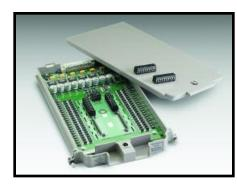
The Model 7710 plug-in module offers 20 channels of 2-pole or 10 channels of 4-pole relay input that can be configured as two independent banks of multiplexers. The relays are solid state, providing long life and low maintenance. Solid-state relays usually have 100 times longer life than mechanical relays. It is ideal for long-term data logging applications as well as for demanding high-speed applications.
