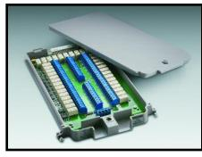
The Model 7708 plug-in module offers 40 channels of 2-pole or 20 channels of 4-pole multiplexer switching that can be configured as two independent banks of multiplexers. The built-in CJC sensors automatically linearize thermocouples, making the Model 7708 ideal for RTD, thermistor, and thermocouple temperature applications. It is also well suited for mixed-signal measurement applications that require multipoint monitoring, such as environmental stress screening.
