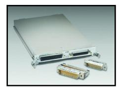
The Model 7701 plug-in module offers 32 channels of 2-pole or 16 channels of 4-pole multiplexer switching. Its 32 channels can be configured for common-side 4-wire ohms. They can also be configured as two independent banks of multiplexers. It is ideal for RTD or thermistor temperature applications.
