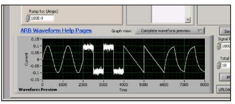
Figure 4. The Model 6221 and the free start-up control software supplied make it easy to create complex waveforms by adding, multiplying, stringing together, or applying filters to standard wave shapes.
