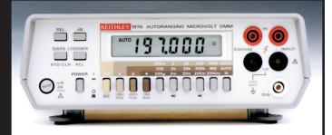
The Model 197A is a lightweight, portable DMM with a battery pack option. It combines 5½-digit resolution (on a 220,000-count display) with 1 $\mu$ V, 1nA, 1m $\Omega$  sensitivity. Basic DCV accuracy is 0.011%.
