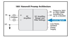
The Model 1801 can measure temperature differentials accurately using a variety of sensors, including type J, K, T, E, R, S, and B differential thermocouples. Users may also enter a specific  $\mu$ V/°C value, making it possible to measure temperature using thermopiles. Thermistor measurements can be made by inputting a constant current to the sensor, then calculating temperature from the resulting  $\mu$ V/°C output.
