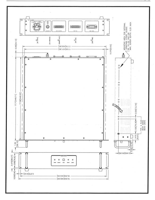
Figure 1-4, IF488, GPIB Interface Unit
